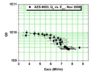
Figure 2: Q<sub>0</sub>-E<sub>acc</sub> curve of a 9-cell cavity.
