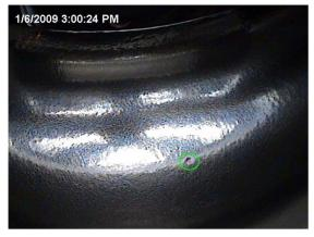
Figure 6: A defect found on a stiffening ring welding area in cell 2 at 30° that seems responsible for FE in  $\pi$  mode.
