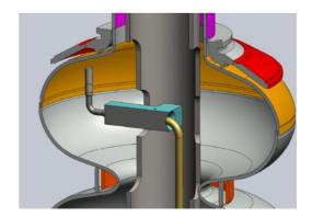
Figure 5: Cavity inner surface inspection using a video scope [8].
