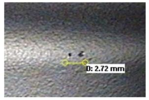
Figure 7: Defects found on the bottom surface of cell 2 at  $190^{\circ}$  that seem to be responsible for the heating in  $7/9\pi$  mode.
