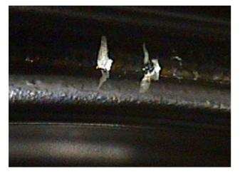
Figure 8: Two scratches found on the iris between cells 6 and 7 at 70° that seem to be responsible for the heating in  $6/9\pi$  mode.
