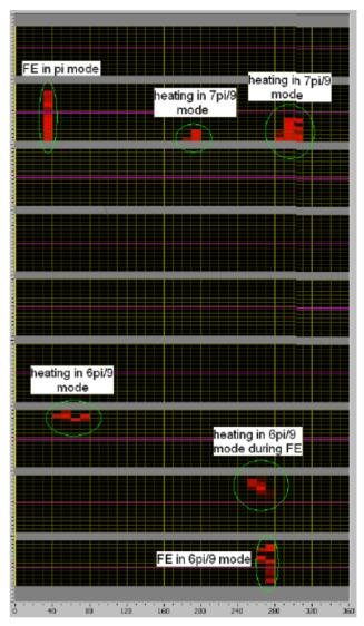
Figure 4: A summary of 2D temperature maps taken at different cavity modes. The magenta line shows the equator of each cell. FE denotes field emission.
