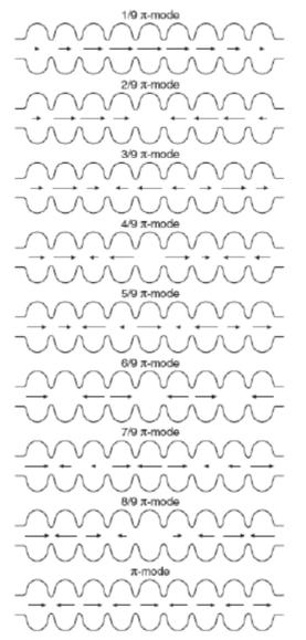
Figure 3: Cavity modes. The direction and length of an arrow represent the direction of electric field and strength at an instant, respectively [7].
