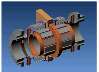
Figure 3. One example of the improved HOM load in the existing bellows assembly.
