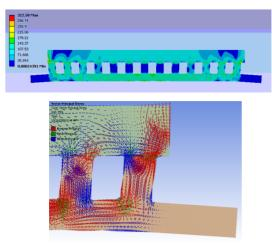
Figure 2. ANSYS calculation showing conceptually how the displacement of posts isolates the difference in thermal expansion of the copper and ferrite, thereby reducing the tensile stresses in the ferrite.
