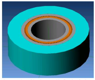
Figure 5. View of brazing assembly fixturing for inner and outer cylinders of ferrite using a suitable keeper ring to prevent the outer ferrite from being in tensile during the brazing process. After cool down, the inner ring is not brazed but held in compression by the extruded copper inner core.
