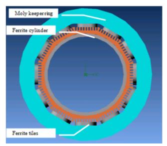
Figure 4. Top view of fixturing for a single braze cycle. The process brazes the outer ferrite tiles and places the inner ferrite cylinder in compression without braze material.
