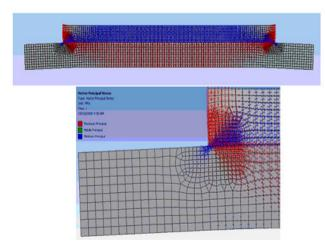
Figure 1. ANSYS calculation of a ferrite material brazed to copper. Maximum Principle stress is shown in red, the tensile stress. The minimum principle stress, compression, is shown in blue.
