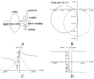
Figure 2: Calculated signal, where dashed curves indicate signal from the cavity, and solid curves indicate the superposition of cavity signal and direct coupling signal.
