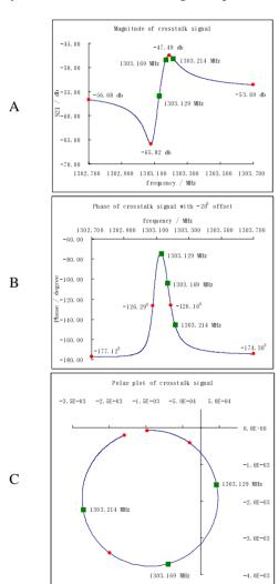
Figure 1: Typical crosstalk signals measured at room temperature. A, B, and C are the magnitude, phase, and polar plot, respectively.
