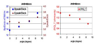
Figure 2: Peak surface fields (left) and R/Q (right) as a function of the wall angle for 60mm of the equator radius.
