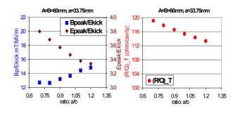
Figure 4: Peak surface fields (left) and R/Q (right) as a function of the iris ellipse aspect ratio a/b. The wall angle is 0 degree and the equator radius is 60mm.
