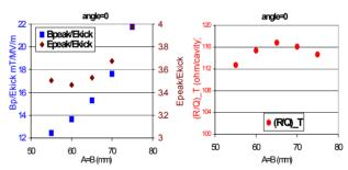
Figure 3: Peak surface fields (left) and R/Q (right) as a function of the equator radius A=B for 0 degree of the cavity wall angle.
