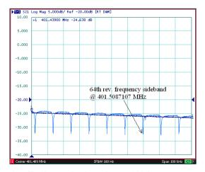
Fig. 4: Effective cavity impedance, 100 kHz span around the frequency of 401.489 MHz.
