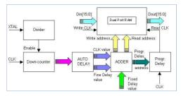
Fig. 5: Automatic Delay Compensation. Block diagram.
