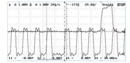
Fig. 6: Read data of RAM are synchronized to the read clock (bottom) changing just before the end cycle (top).
