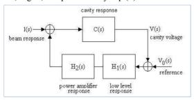
Fig. 1: Closed loop response for a cavity feedback system.
