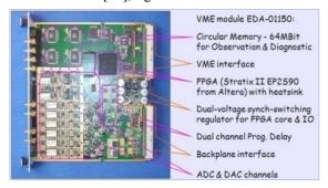
Fig. 7: LHC 1-T Feedback, VME module EDA-01150.
