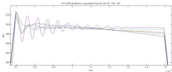
Figure 10: Total FLASH field as a function of the feedback control proportional gain.
