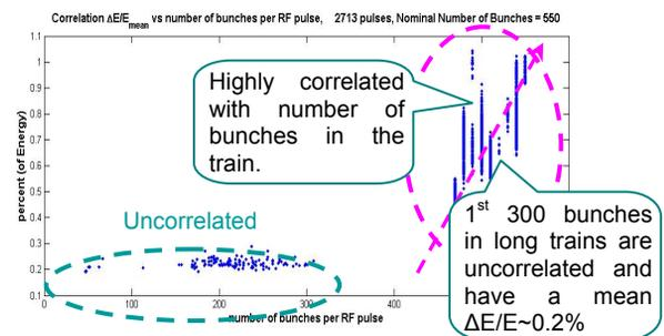
Figure 6:  $\Delta E/E$  vs. bunch train length correlation.
