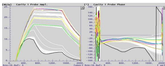
Figure 9: Cavity quench.
