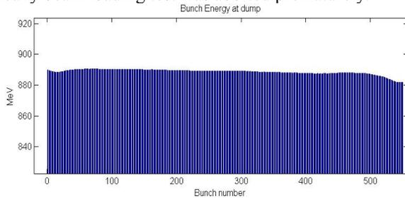
Figure 2: Energy measured by the spectrometer at the dump.
