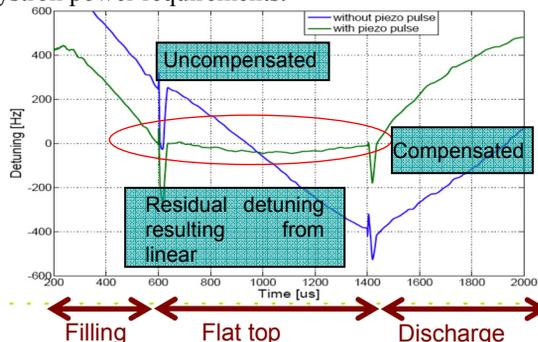
Figure 11: Resonant frequency control using piezoelectric actuators.
