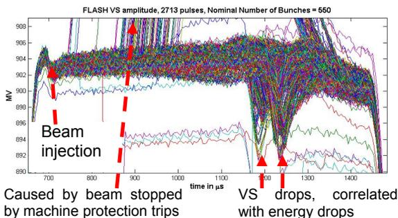
Figure 7: Amplitudes of FLASH gradient for 2713 over imposed pulses.
