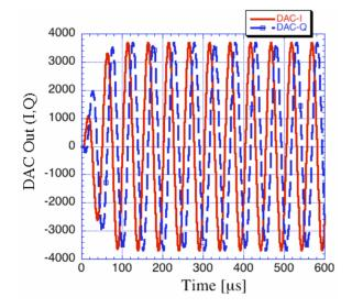
Figure 6: I and Q components of the DAC output when 20-kHz detuning is given.
