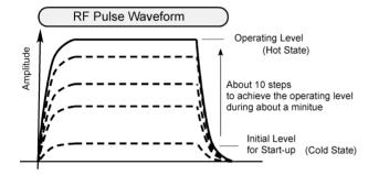
Figure 2: Amplitude is increased step by step for the cavity start-up (slow start). The tuner is controlled during this sequence.
