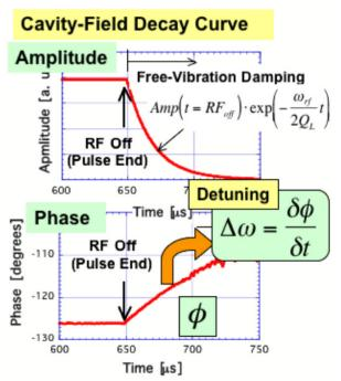
Figure 5: The Q-Value and the detuning of the cavity are obtained from the field decay curve
