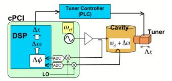
Figure 3: Cavity tuner control with DSP..
