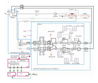
Figure 1: FPGA block diagram of the digital FB and FF control system for the J-PARC linac LLRF.
