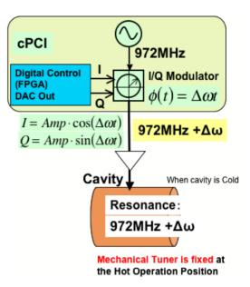
Figure 4: The phase is rotated with the IQ modulator in detuned frequency.
