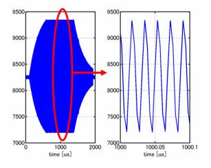
Figure 9: Raw data at 270MHz.
