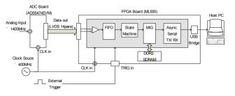
Figure 1: Block diagram of high-speed data acquisition system.
