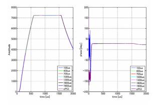
Figure 6: Overall amplitude and phase waveforms (270.83 MHz and IF scheme (cPCI)).
