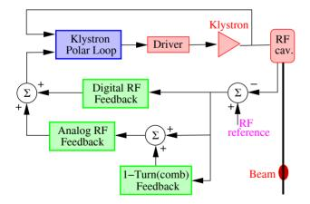
Figure 1: Simplified LHC RF block diagram.
