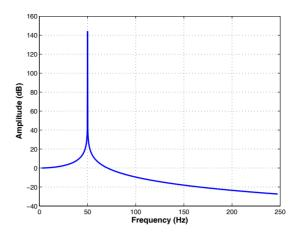
Figure 3: Beam Transfer Function
