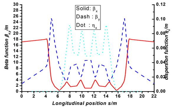
Figure 1: Twiss and dispersion function of FBA
