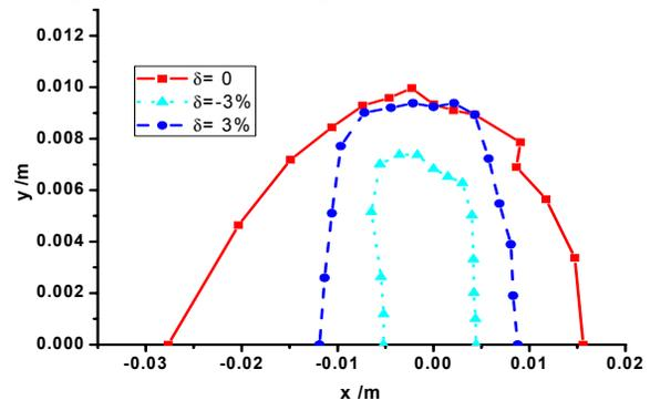
Figure 4: 1000-turn dynamic aperture of QBA
