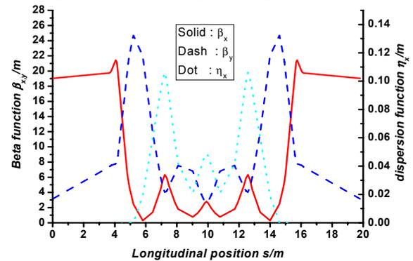
Figure 3: Twiss and dispersion function of QBA
