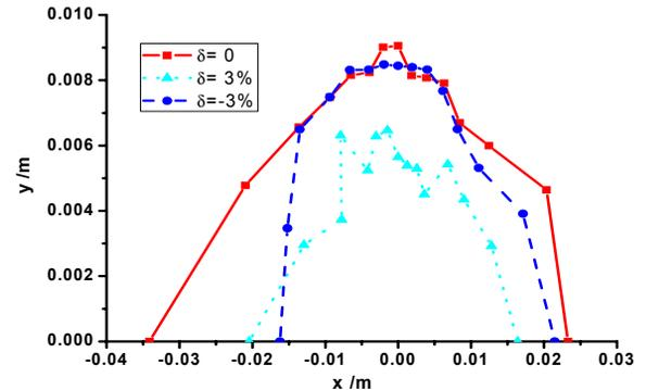
Figure 2: 1000-turn dynamic aperture of FBA
