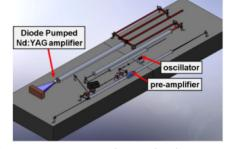
Figure 5: 10 J, 120-Hz interaction laser system.
