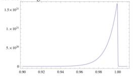
Fig. 2 Typical on-axis spectral brightness (see Table 1). The vertical axis is the number of photons/(s x  $mm^2$  x  $mrad^2$  x 0.1% bandwidth); the horizontal axis is normalized to the Compton scattering energy, 2.22 MeV.
