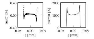
Figure 2: Longitudinal phase space and current distribution after bunch compression, acceleration to 1.7 GeV, and passage through a 3-stage beam spreader with a low value of  $R_{56}$ . The tail is on the right.
