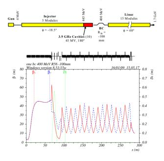
Figure 1: Schematic diagram and lattice functions of the single-stage bunch compressor.
