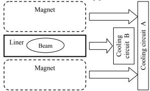
Figure 1: Schematic of the undulator cold mass. The superconducting coils are thermally separated from the liner and are independently cooled.
