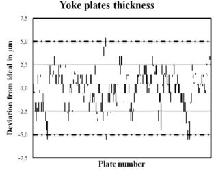
Figure 4: Manufacturing accuracy of 204 yoke plates, on the vertical axis is shown the deviation with respect to the ideal thickness of 7.5 mm.
