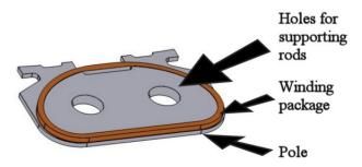
Figure 3: 3D model of one of the 408 plates constituting the two magnet yokes. Each plate includes a pole and a superconducting coil winding.
