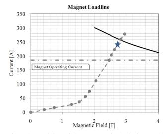
Figure 2: Load line of the magnet. The dashed curve is the load line of the magnet which is iron dominated at low fields. The dot-dashed line represents the operating current of the magnet. The star indicates the maximum operating current of a 3-periods prototype tested in LHe.
