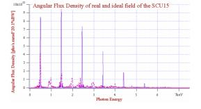
Figure 4: Comparisons of the angular flux density for measured and ideal field. The ideal field is 1.3521 T and the period length is the average measured value of 15.007 mm. The beam energy and beam current are 1.5 GeV and 0.2 A respectively.
