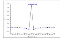
Figure 6: Peak field changes with an additional coil wound around the 21<sup>st</sup> pole with a current of 59 Ampere.
