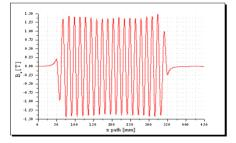
Figure 2: Measured field of the SCU15 along the beam axis using the Hall probe sensor.
