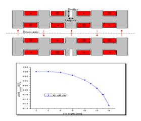
Figure 8: Cross-section of the SCU15 with inserted slit into backside of the poles (upper) and varying depth of inserted slit into the poles as a function of the changes in field (lower).
