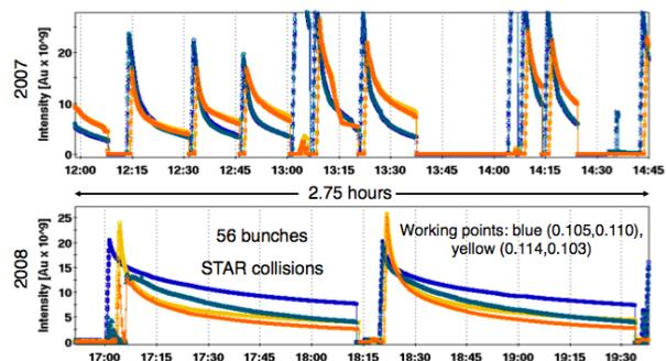
Figure 1: Comparison of 2007 and 2008 beam lifetimes at  $\sqrt{s}=9.18$  GeV/n. Sextupole reversal and elimination of octopoles clearly improved beam lifetime.
