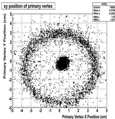
Figure 3: Reconstructed vertex locations of  $\sqrt{s}=9.18$  GeV/n collisions at the STAR experiment during the 2008 run. Both beam-beam and beam-beampipe collisions are clearly visible, consistent with the beampipe inner diameter of 76mm. (Figure courtesy of the STAR collaboration, private communication.)
