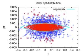
Figure 1: Initial longitudinal particle distribution for the injection energy case; in red are particles which will be lost when kicking at the nominal vertical betatron frequency and maximum kick reduced by a factor 10 together with the separatrix (cyan).
