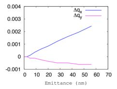
Figure 6: Tune variation vs. particle emittance (by FFT of Turn-By-Turn data, luminosity optics with errors).
