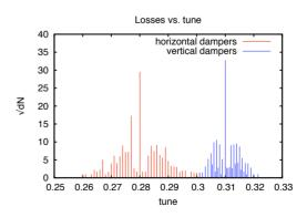
Figure 5: Number (sqrt) of lost particles vs. excitation frequency
