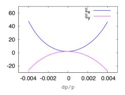
Figure 4: Chromaticities vs. momentum (MAD-X, injection optics with errors).
