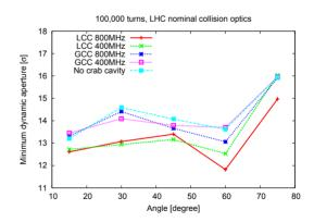
Figure 2: Dynamic aperture for nominal LHC optics.
