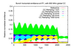
Figure 5: Emittance growth from CC ramping.
