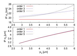
Figure 7: (top): Vertical beam size  $\sigma_y$  at the IP versus horizontal emittance for three different orders:quadrupolar, octupolar and dodecapolar. (bottom): Horizontal beam size  $\sigma_x$  at the IP versus horizontal emittance for the same orders.
