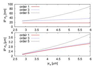
Figure 3: (top): Vertical beam size  $\sigma_y$  at the IP versus horizontal emittance for three different orders: first, third and fifth. Clearly the fifth order amplify dramatically the beam size
