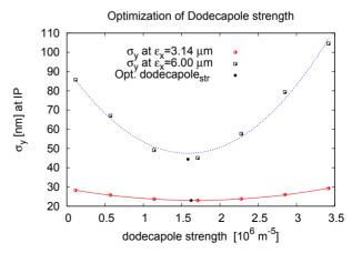
Figure 4: Qualitative study for the optimization of the dodecapole strength at lower and higher  $\epsilon_x$ . Keeping the ultralow beta lattice design unmodified. The black solid points mark the minimum  $\sigma_y$  at the IP for both cases.
