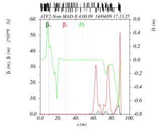
Figure 2: Nominal  $\beta_x$ ,  $\beta_y$  and horizontal Dispersion  $D_x$  functions for the ATF2 ultra-low  $\beta$  proposal. It should be noted the present symmetry around 70m concerning  $\beta_y$ .
