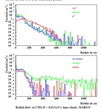
Figure 5: Radial distributions of particle fluxes (E>20 MeV) at z=22.6 m from IP5 (R) for "elastic beam-gas".
