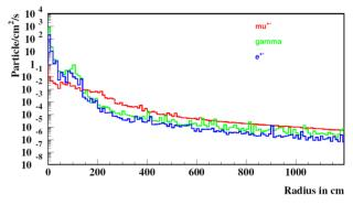
Figure 6: Radial distributions of particle fluxes (E>20 MeV) at z=22.6 m from IP for "inelastic beam-gas" [2].
