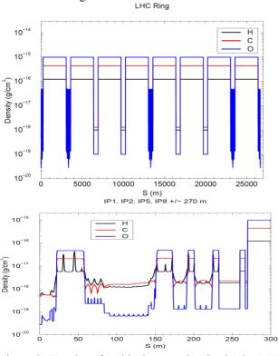
Figure 2: Density of residual gas molecules in the LHC ring (top) and interaction regions (bottom).
