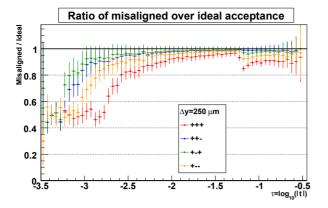
Figure 5: Ratio of the acceptance determined for different configuration of quadrupole misalignement over the ideal one.
