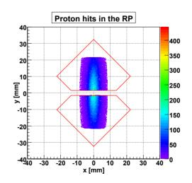
Figure 2: Proton hits distibution in the RPs. The two red diamond shape represents the upper and the lower part of the RPs.
