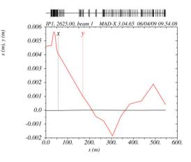
Figure 4: Displacement of the closed orbit for the +++ configuration.
