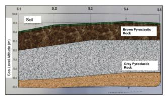
Figure 2: Ground cross section.
