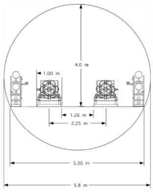
Figure 8: Storage rings tunnel occupancy second scenario.
