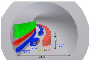
Figure 7: Storage rings tunnel occupancy.
