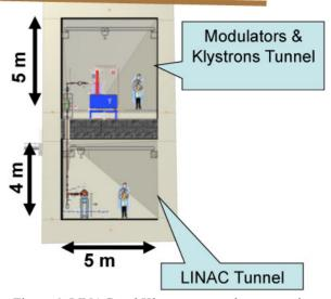
Figure 6: LINAC and Klystrons tunnel cross section.
