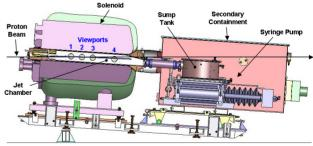
Figure 1: Vertical cross-section of MERIT equipment.
