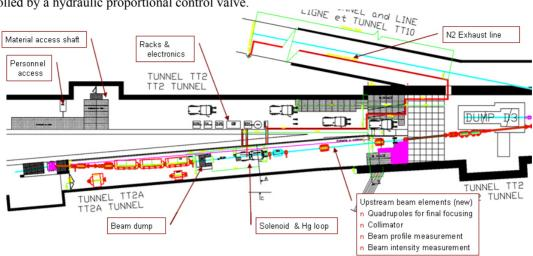
Figure 2. MERIT experimental layout in CERN TT2/TT2A tunnels.
