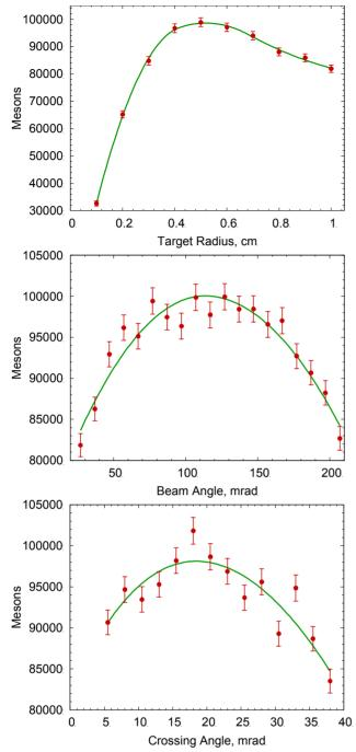
Figure 3: Meson production as a function of target radius (top), proton beam angle (middle), and beamtarget crossing angle (bottom). Data points represent mesons generated from  $10^5$  incoming 50GeV protons. Curves are least-squares fits to this data.
