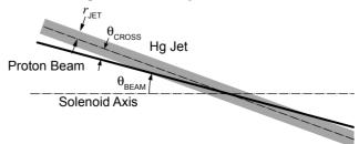
Figure 2: The mercury jet target geometry.
