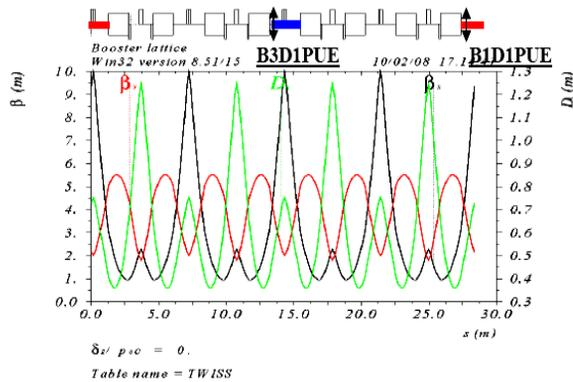
Figure 3: The horizontal (black) and vertical (red) beta functions, and dispersion function (green). Positions of B1D1PUE and B3D1PUE are indicated by vertical arrows (black).
