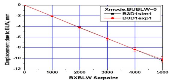
Figure 7: Maximum excursion of the difference orbit vs. BXBLW setpoint at B3D1PUE while BUBLW is OFF.
