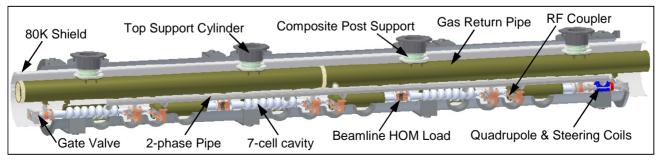
Figure 1: A cut-away CAD model showing the main features of the ERL Linac cryomodule.
