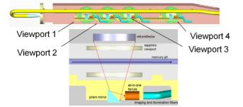
Figure 2: Details of the optical diagnostic system. The Hg jet was photographed by high-speed cameras at view-ports 1, 2, 3, and 4 as it streamed from left to right. The center of the overlap of the Hg jet and the proton beam was at view port 2, and the aftermath of the interaction was viewed at view ports 3 and 4.
