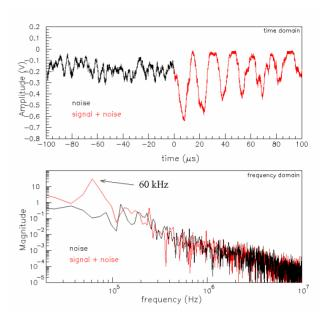
Figure 4: VISAR signal as a function of time (top) and corresponding frequency spectrum (bottom). An arrow indicates the position of characteristic signature of the longitudinal expansion of the tungsten wire.
