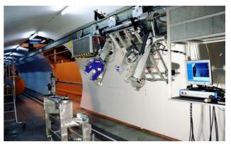
Figure 2: TIM with remote collimator alignment measurement module during testing in tunnel mock-up
