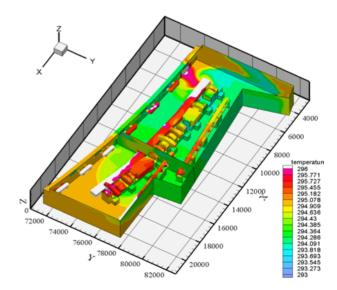
Figure 4: Simulated temperature distribution in the storage ring tunnel.
