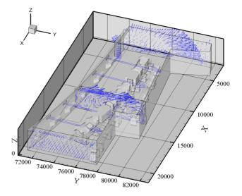
Figure 3: Model of 1/24 storage ring and simulated air velocity vectors.
