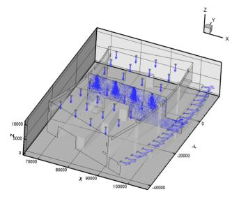
Figure 5: Model of 1/12 experimental hall and simulated air velocity vectors.
