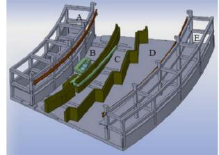
Figure 2: 3D schematic view of one 1/12 of the TPS storage building.
