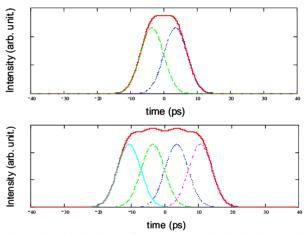
Figure 4. Simulations of two (non-optimized) laser pulse stacking cases for use at the AWA with an a-cut,  $\alpha$ -BBO crystal.
