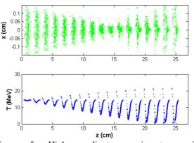
Figure 5. High gradient experiment, maximum transmission case. Top: transverse profile; Bottom: Longitudinal phase space. The results are shown at 50ps intervals; z is the axial position along the structure.
