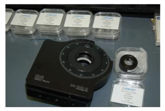
Figure 3. Crystals and rotational mount used to lengthen the bunch length of the AWA beam so that the bunch length can match the wavelength of the DLA structure in the transformer ratio enhancement experiment [5].
