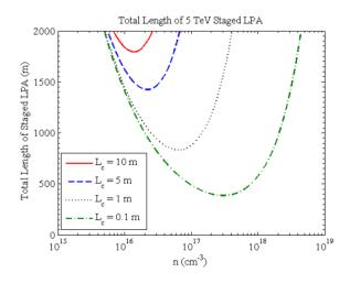
Figure 2: Main single-linac length versus plasma density  $n_0$  for several laser in-coupling distances  $L_c$ ,  $E_b = 5$  TeV and  $a_0 = 1.5$  [6]
