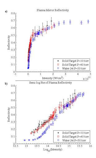
Figure 4: a) Reflectivity of plasma mirror. b) Semi-log plot of reflectivity.
