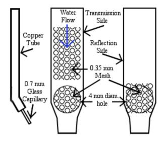
Figure 3: Schematic of water jet and guiding structure.
