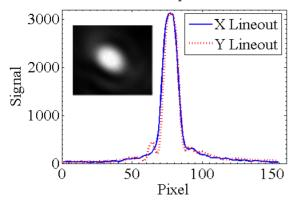
Figure 5: Near field image of the mode of TREX laser reflected from water jet at  $\approx 50$  torr pressure.
