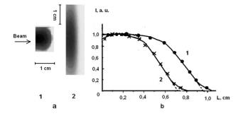
Figure 4: a) - change of darkness density of glass plate, caused by irradiation with relativistic electron bunches (1) – at entrance and (2) - at exit of dielectric structure; b)distribution of darkness density along thickness of a glass plate in direction of beam propagation.
