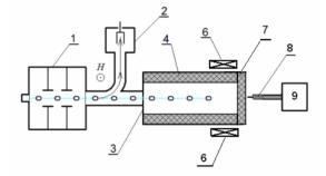
Figure 1: Scheme of the installation: 1-electron accelerator, 2-magnetic analyzers, 3-diaphragm, 4-dielectric plates, 5-rectangular copper waveguide, 6-deflecting magnets, 7-Teflon seal, 8-RF-probe, 9-oscillograph
