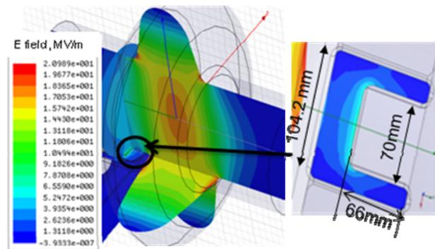
Figure 2: HFSS plot of the electric field intensity in the waveguide to beam pipe coupling aperture. Fields are normalized to 2.4MV accelerating voltage.
