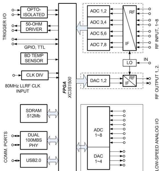
Figure 1: Functional diagram of the field controller module.
