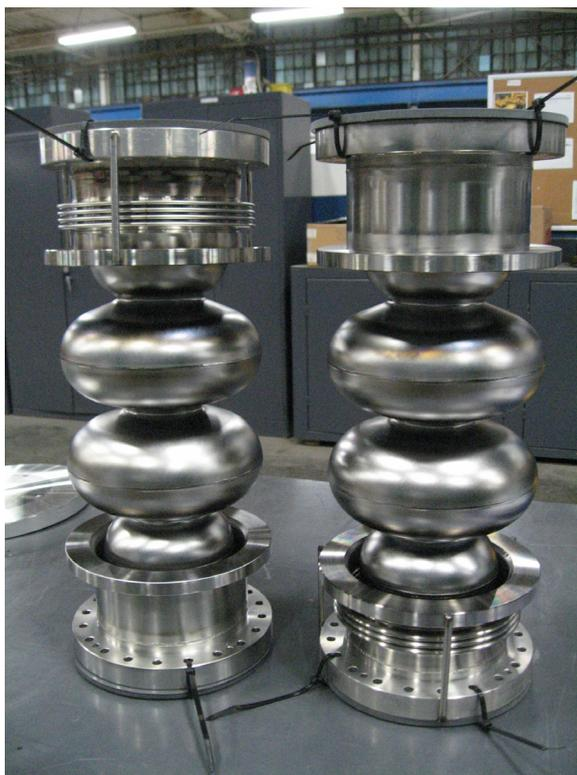
Figure 3: 1500 MHz two-cell niobium cavities with SS helium vessel end spoils.
