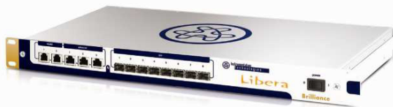
Figure 1: Libera BPM electronics with RocketIO used to implement the ‘Diamond Communication Controller’ [7]
