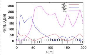
Figure 1: IR layout and Twiss functions.
