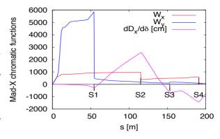
Figure 2: IR MAD-X chromatic functions,  $W_z = \sqrt{(A_z^2 + B_z^2)}$ , and sextupole locations. The sextupole S3 at 150 m corrects  $dD_x/d\delta$ .
