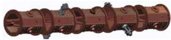
Figure 1: Engineering model of the five-segment RFQ.
