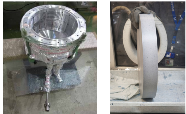
Figure 2: (a) 35 cm LH 2 absorber body and (b) the 63 mm LiH absorber .
