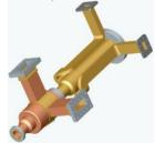
Figure 6: RF structure for second harmonic power source.
