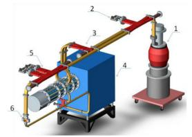
Figure 5: Layout of dual-frequency RF source, shown feeding a bimodal test cavity. 1 – S-band klystron; 2 – variable power splitter; 3 – 3-dB hybrid splitter; 4 – 250-kV electron gun tank; 5 – variable power splitter and phase shifter; 6 - bimodal test cavity. Gray structure attached to gun tank is the magnetic circuit, within which the two-cavity source is positioned.
