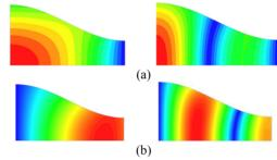
Figure 1: (a) The electric field map and (b) the magnetic field map for 2.856 GHz  $TM_{01}$  and 5.712 GHz  $TM_{02}$ modes.
