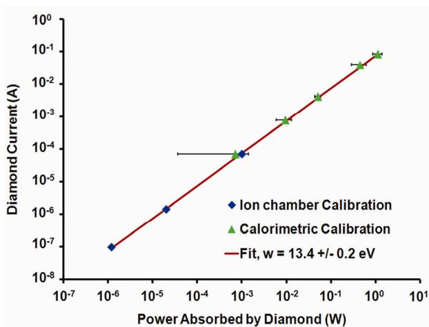
Figure 4: Diamond detector flux linearity
