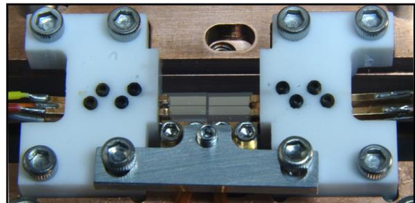
Figure 1: NSLS X25 white beam position monitor (BPM)
