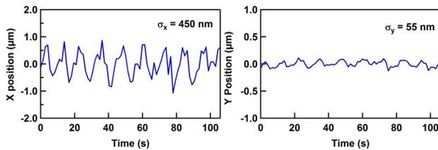
Figure 6. X25 BPM position noise measurement
