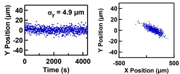
Figure 9: Long term vertical stability (left) and x-y correlation of beam motion (right)
