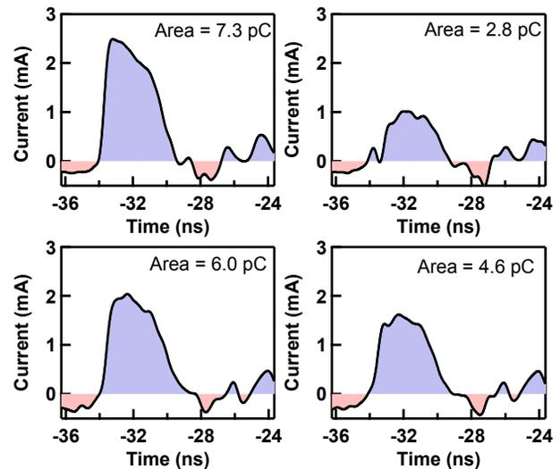
Figure 8: Integrated charge from a single x-ray pulse on the four pads of a quadrant detector
