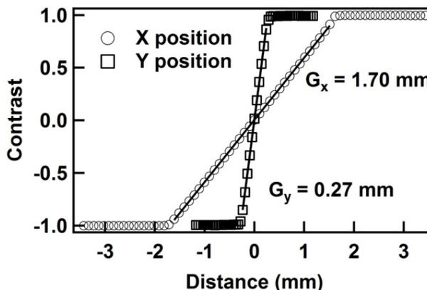
Figure 5: Positional calibration of the X25 BPM
