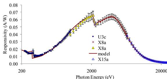
Figure 3: Diamond detector spectral response
