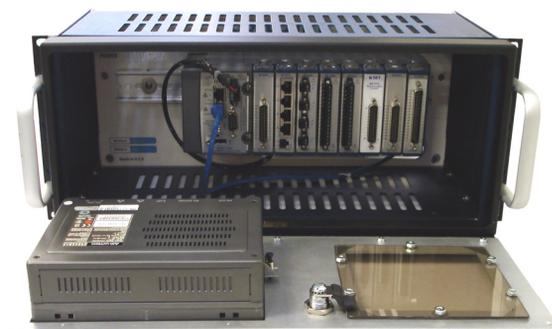
Figure 4: cRIO Crate Mounting in Chassis Unit.
