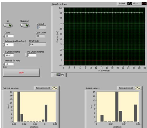
Figure 5: Limit switches repeatability test.
