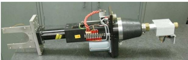
Figure 11: MP-11 wire scanner.
