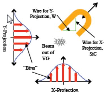
Figure 1: wire scanner basics diagram.
