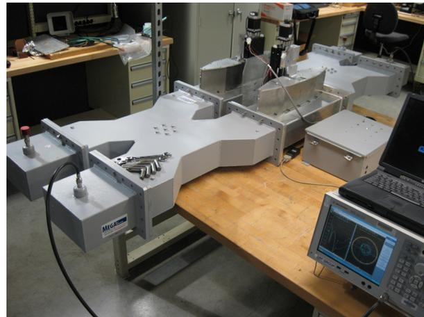
Figure 3: Low power bench measurement of a vector modulator setup.
