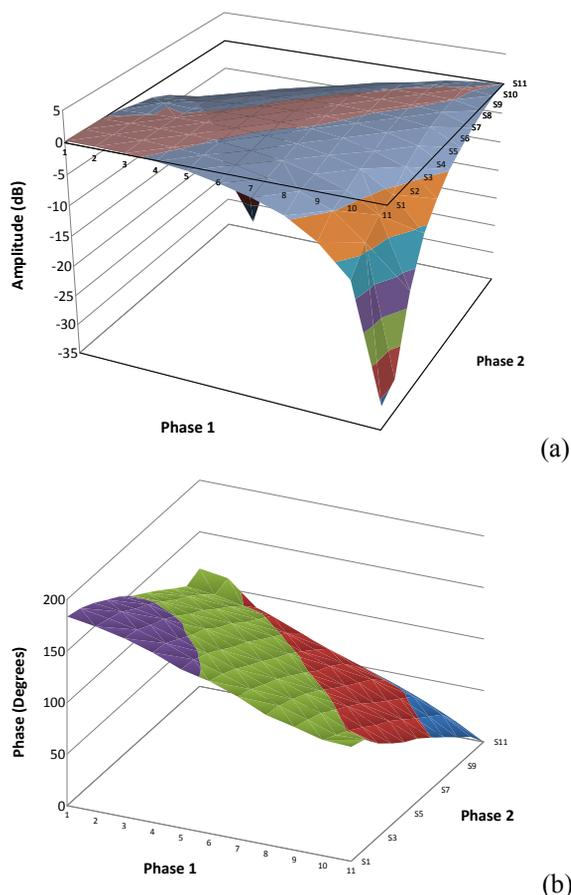
Figure 4: Low power bench measurement of a vector modulator setup. (a) Amplitude, (b) Phase.
