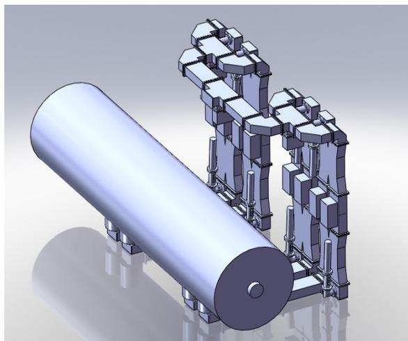
Figure 1: Layout of four-way waveguide power splitting system for a four-cavity cryomodule test.
