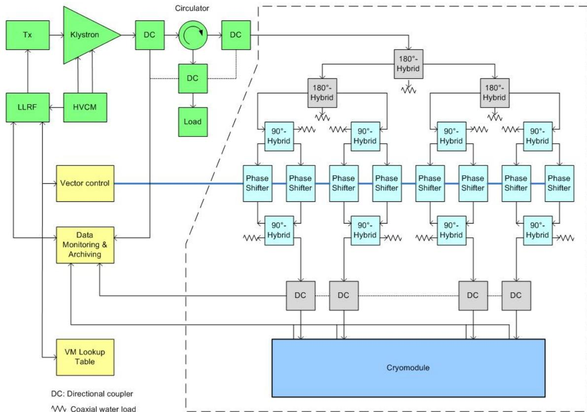
Figure 2: High power RF distribution system using waveguide vector modulators being implemented for testing up to four cavities in a cryomodule simultaneously.
