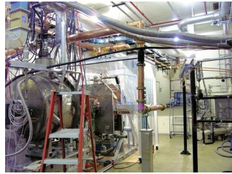
Figure 5: MTA enclosure showing 5-T solenoid in foreground and 201-MHz cavity behind it.
