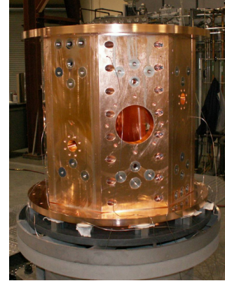
Figure 5: Brazed segment of the prototype cavity.
