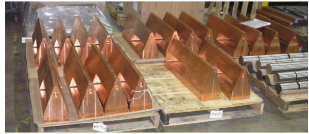
Figure 4: Vane blocks after pre-brazed machining.
