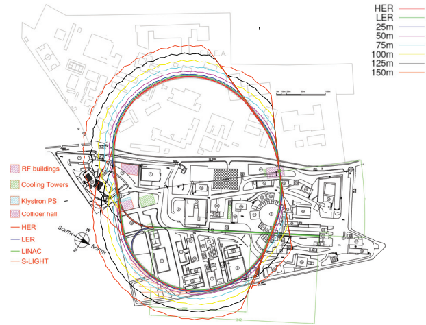
Figure 4: All possible bend magnet photon beam line location with different contour lines showing the distance to the source point.
