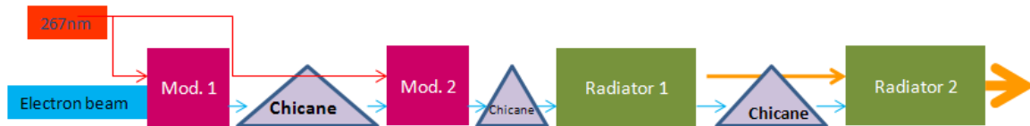
Figure 1: Using the fresh bunch technique [4], a radiator following a regular Echo enabled FEL [5] can deliver high power radiation pulses of soft x-rays. The EEHG part consists of two 2.25 m modulators, each with a period length of 25 cm. The EEHG-radiator has a period length of 4.5 cm and consist of two undulators each 4.5 m long. The second radiator consists of 8 undulators, each 4.5 m long with a period length of 4.5 cm.
