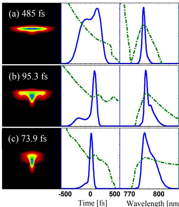
Figure 2: Each experimental FROG result is a row in the figure labelled by the FWHM of the main temporal peak. The three columns, starting from left, show retrieved FROG images, temporal and spectral distributions including phase. Amplitudes (blue) are normalized and phases (green) are plotted from -10 to +10 rad.
