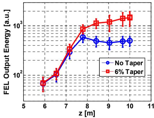
Figure 3: Gain curves with and without tapering.
