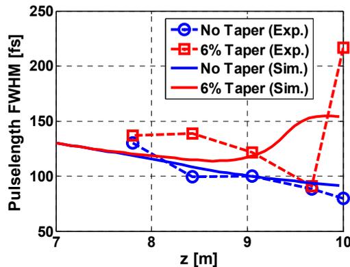
Figure 4: Radiation pulselength (FWHM) evolution along the undulator. Blue and red lines are for non-tapered and tapered cases, respectively. Solid and dashed lines are for simulations and for experiments, respectively.
