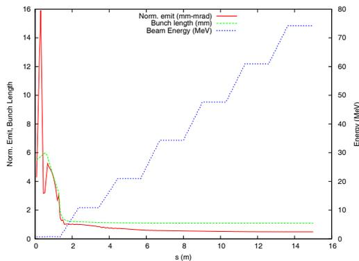
Figure 4: Evolution of full, normalized, RMS  $x$  emittance (mm-mrad, red), RMS bunch length (mm, green) and average beam energy (MeV, blue).
