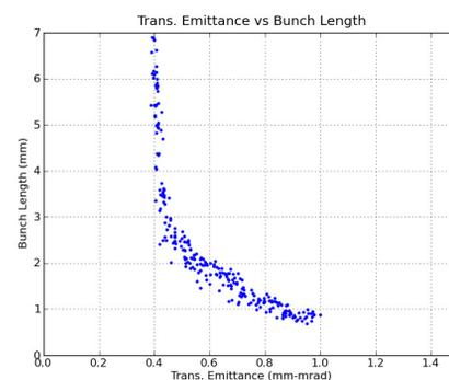
Figure 2: Approximation of the Pareto optimum front (normalized trans. emittance vs bunch length) at the exit of the injector (15 m from the cathode, beam energy of about 70 MeV)
