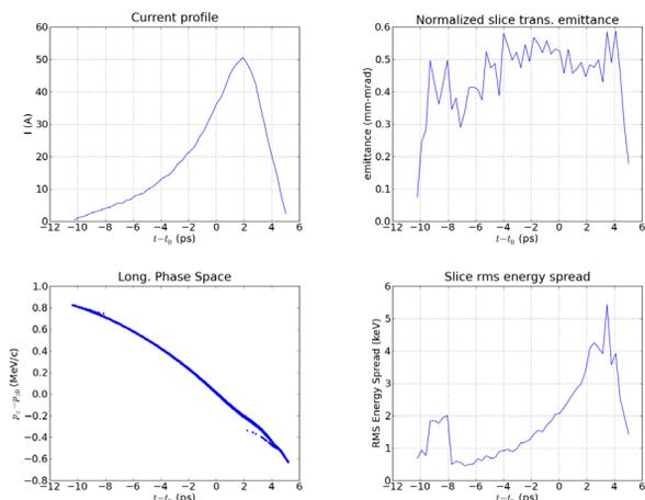
Figure 3: Beam characteristics at the exit of the injector for the design solution. Note that the beam head is located to the right of the beam tail.
