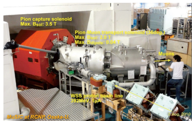
Figure 1: Pion capture and upstream proton beam line.
