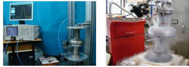
Figure 3: a) RF measurement at 300 K, b) Leak testing & RF measurement at 77K.
